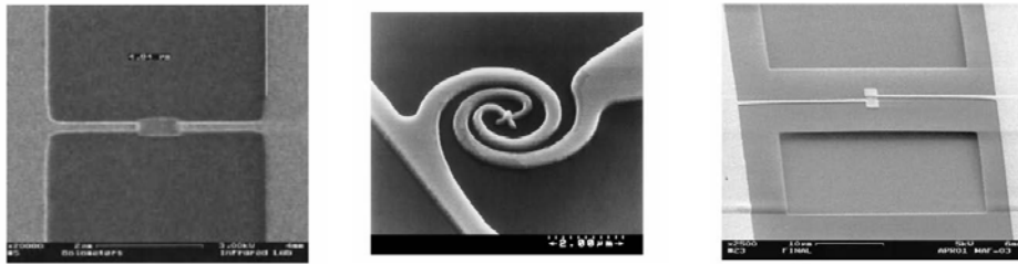
Fig. (2): Different types of optical antennas written by electron beam lithography on Si wafers. We can see a dipole antenna (left), an asymmetric spiral antenna (center), and a patch antenna on a moving bridge (right). The physical mechanism for the transducer is a microbolometer for the left and right antennas, and a MOM diode for the central one.
