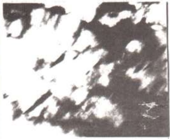
Fig(8) x20K TEM of Alloy(B), Isothermally treated for 20 min at 500 C, coarse carbide precipitates .
