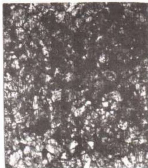
Micrograph (1) x 250 Stainless Steel 18/8 austenitised at 1050 °C and water quenched , (after polarization at 70 °C .)
